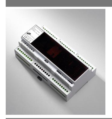
The EBR-DIN-DALIG64 is a Rapid lighting control module designed for controlling 64 addressable DALI devices such as fluorescent or LED lighting ballasts. There are two relays providing a switched live output and a third relay for emergency test. Additionally there is a volt free contact to control external devices.
